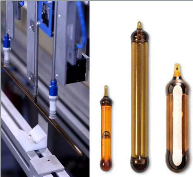
Manufacture of thermally-activated glass ampoules for automatic sprinklers ('e-bulbs')
